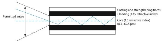
Figure 2. Light Traveling Through a Fibre
